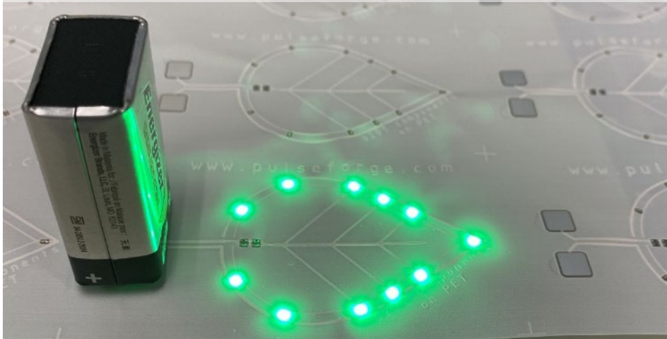
Chip components photonically soldered with SAC 305 alloy on PET flex
